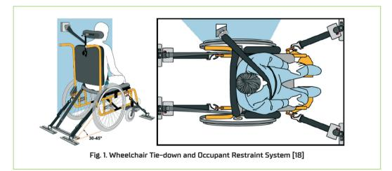
However, this system usually requires a third party to assist with the application of the seatbelt and its routing around wheelchair features. Often this means that a person the wheelchair user is unfamiliar with must enter personal space and physically contact them to apply the seatbelt. This can be uncomfortable for wheelchair users [12].
