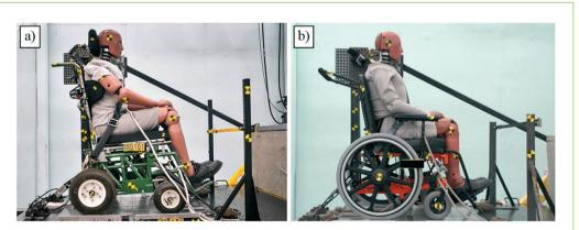
Fig. 4. Example of tiedown/securement system testing; (a) surrogate wheelchair [15], (b) wheelchair frontal-impact testing [8]
