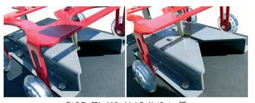
Fig. 2. The EZ Lock Wheelchair Docking System [7]
